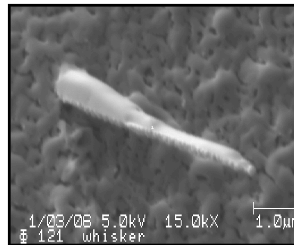
Whisker after 1000 Å sputtering and AES analysis
